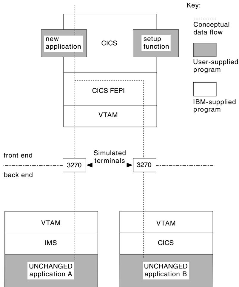
Figure 1. Structure of FEPI and application programs
