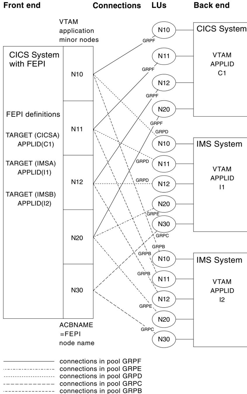
Figure 2. The sample FEPI configuration—a diagrammatic representation
