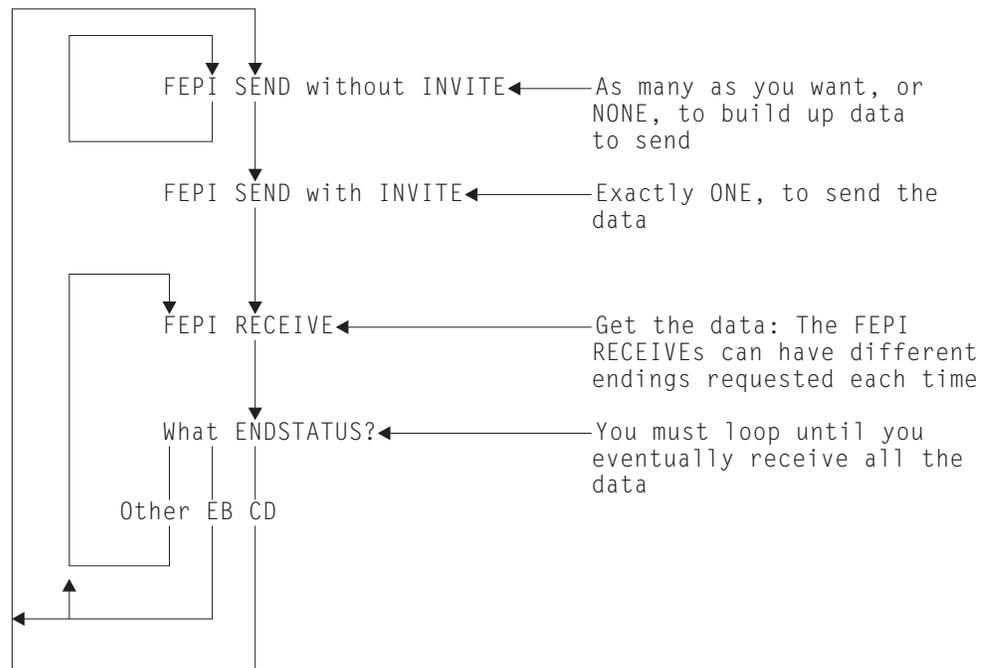
**Note:** The diagram does not show any processing of the data, nor where you might enter, or leave, the loop. This information is explained more fully in Chapter 14, “Application design” on page 119.
