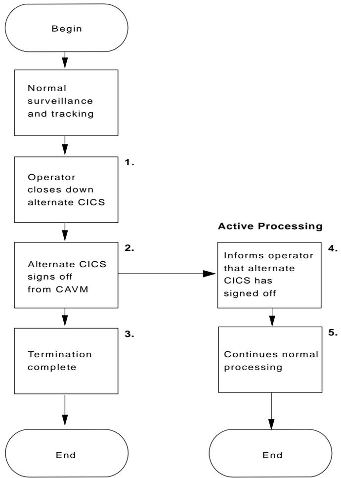
Figure 4. Shutting down the alternate CICS normally
