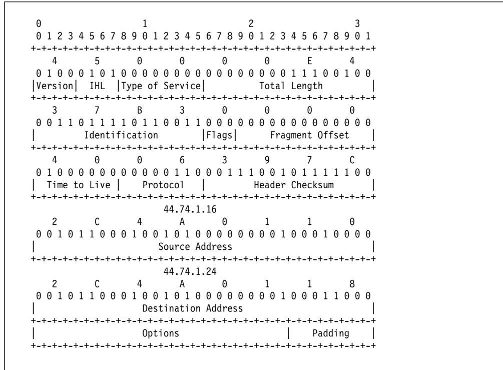
Figure 101. IP Header Format
