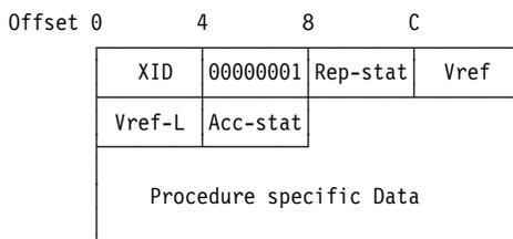
Figure 80. Structure of an RPC Accepted Reply Message
