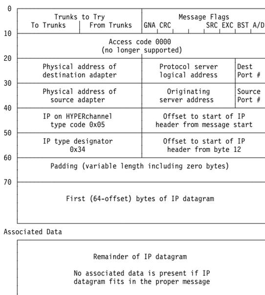
Figure 19. Basic HYPERchannel 16-bit Message Encapsulation
