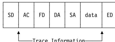
Figure 97. Common Layout of a Token-Ring Packet
