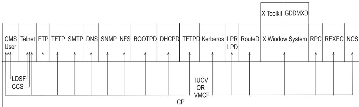
Figure 3. The TCP/IP Layered Architecture for VM
