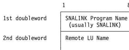
Figure 22. Format of the User Field for an SNA IUCV CONNECT Request
