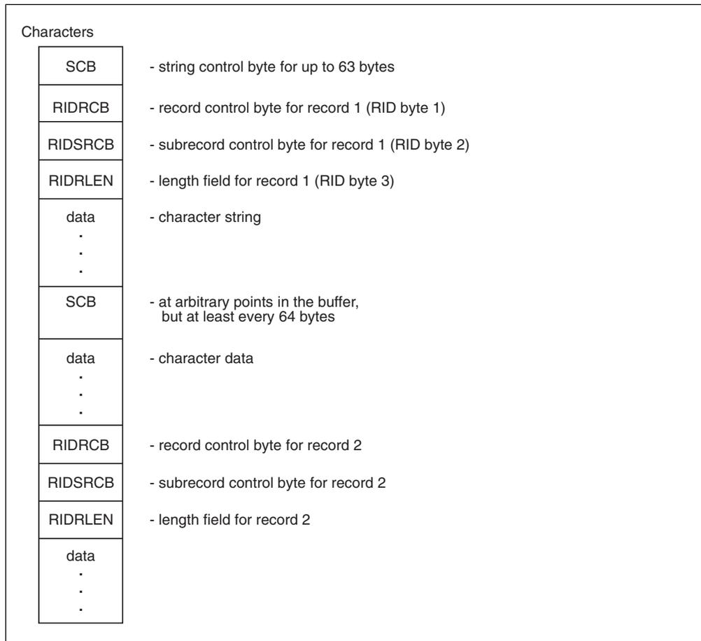
Figure 70. Format of a Transmission Buffer for SNA
