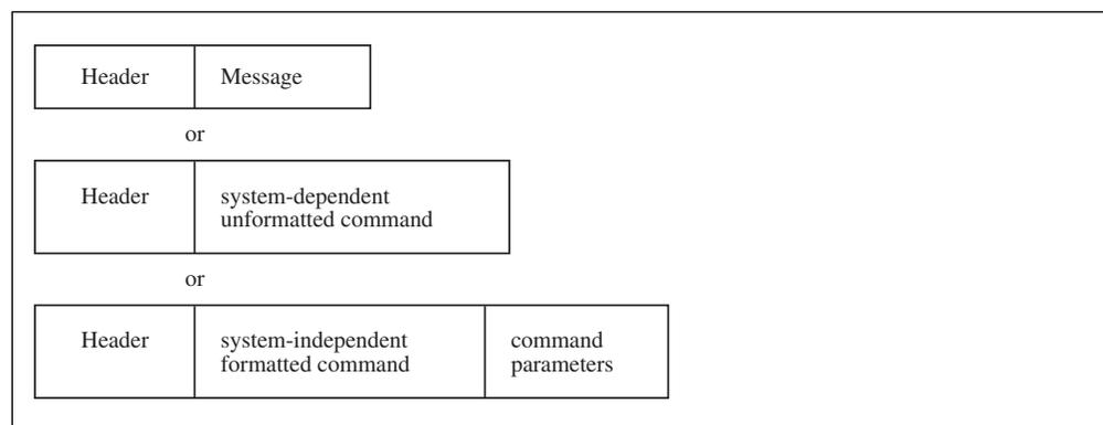
Figure 7. Format of an NMR
