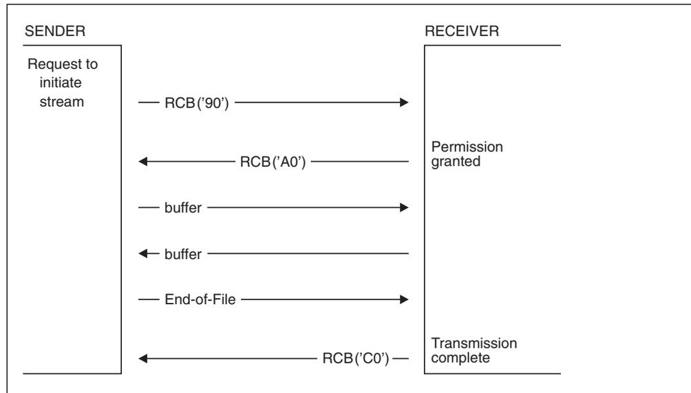
Figure 79. Protocols Used to Transmit a Stream
