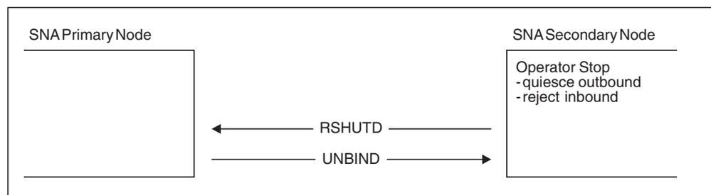
Figure 14. Terminating Processing by an SNA Secondary Node
