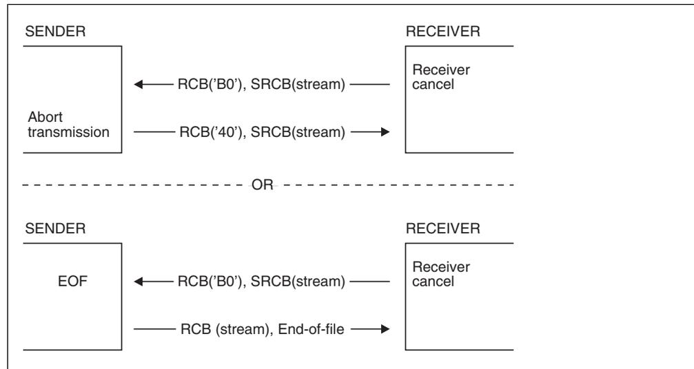
Figure 83. Receiving Node Initiates Stream End
