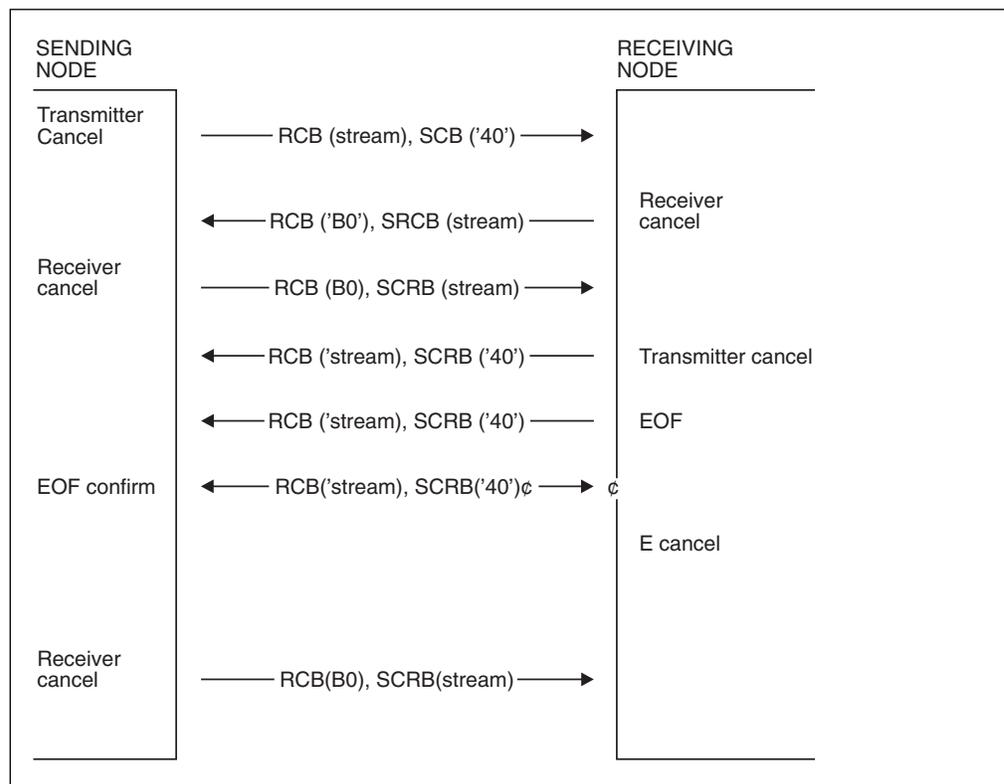
Figure 82. Sending Node Initiates Stream End
