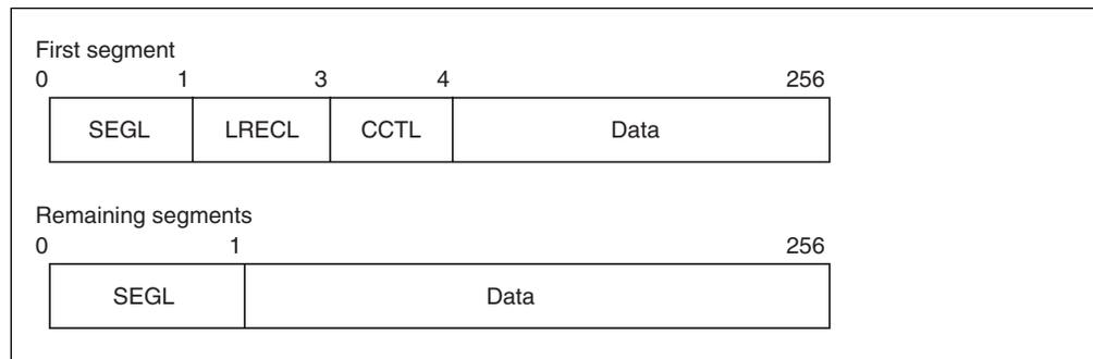
Figure 78. Spanned Data Record With Carriage Control
