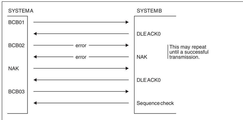
Figure 60. Results of Not Transmitting Null Records.
