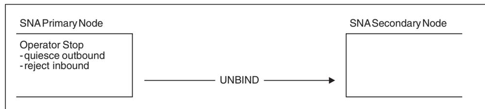
Figure 15. Terminating Processing by an SNA Primary Node
