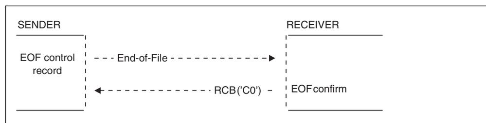
Figure 80. Protocols Used to Transmit a Stream
