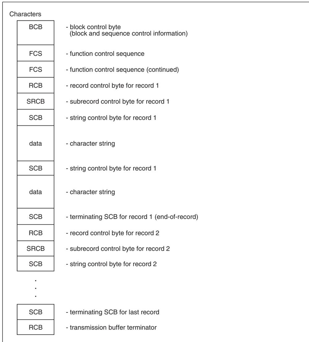
Figure 58. Format of a Transmission Buffer for BSC and CTC
