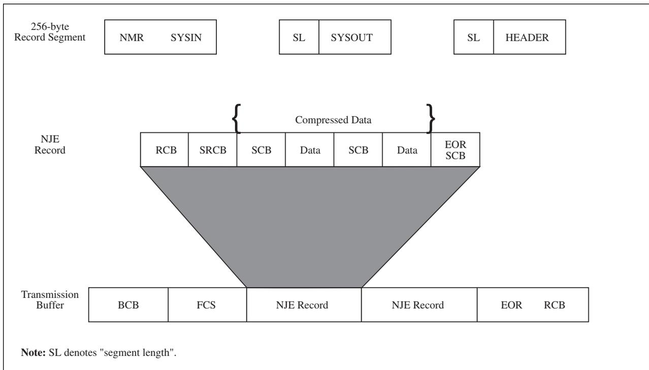
Figure 8. Format of a Transmission Buffer for BSC and CTC Protocols
