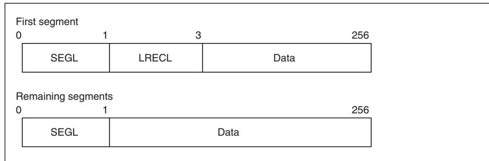
Figure 77. Spanned Data Record
