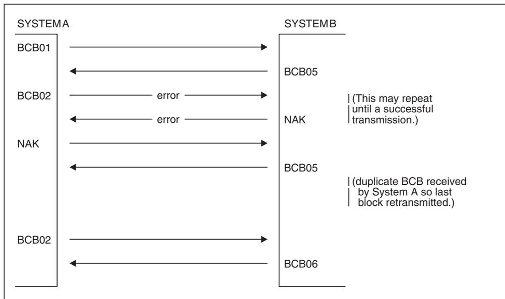
Figure 61. Correct Recovery with Null Records
