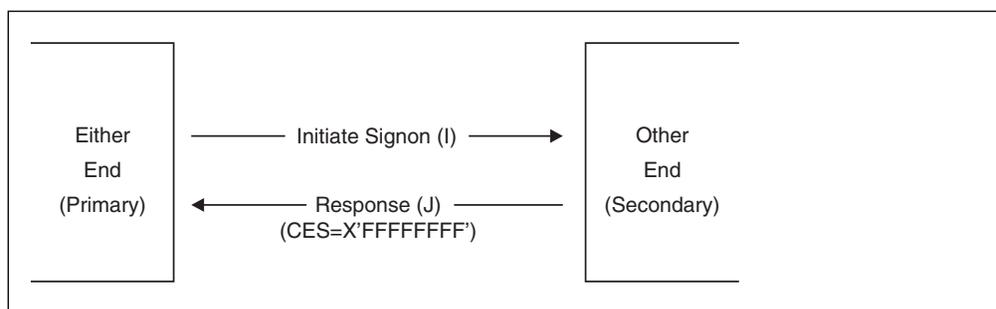
Figure 87. Connection Protocols used by the Non-Path Manager Nodes
