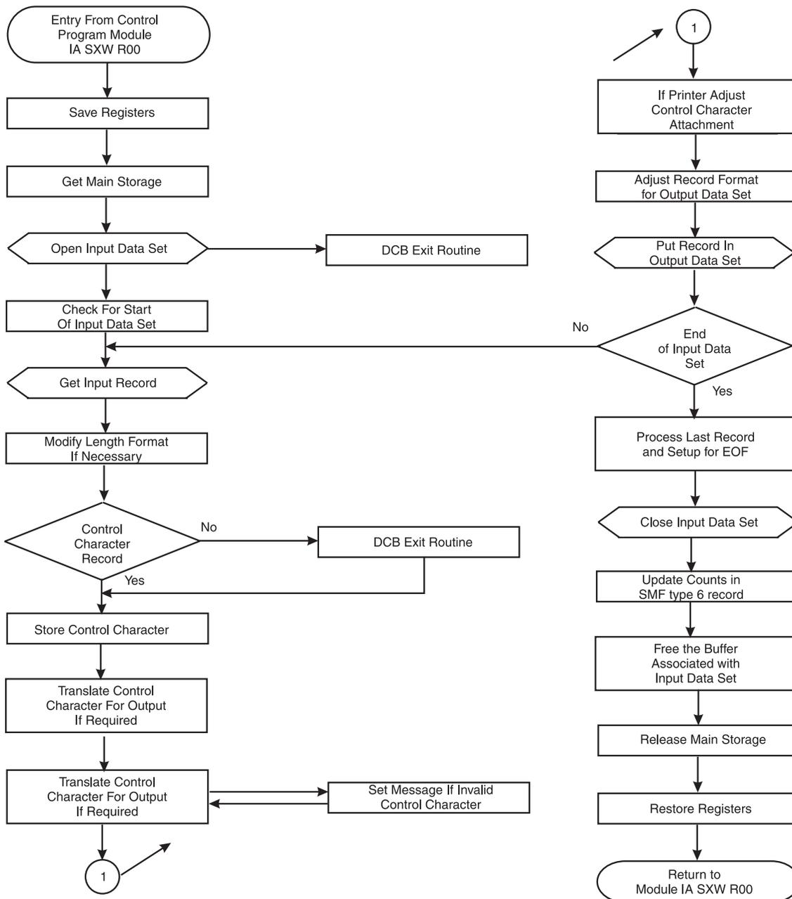
Figure 3. General Flow of IBM's Output Writing Routine
