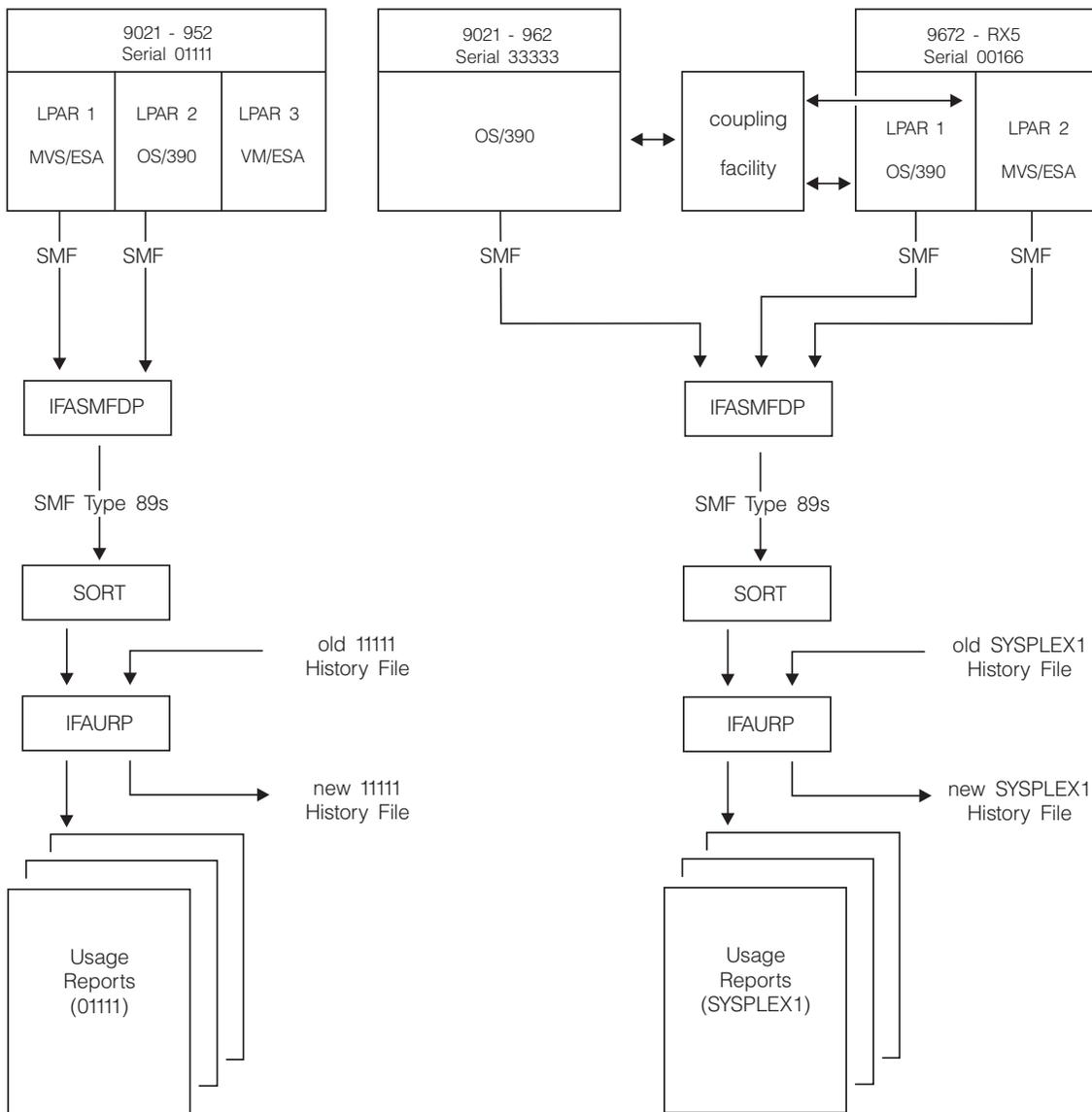
Figure 3. Example of an installation using a separate file for each reporting entity
