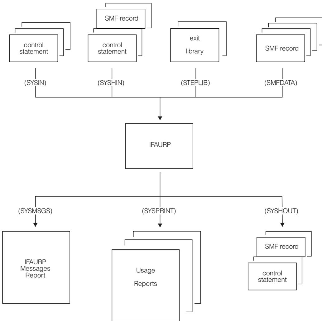
Figure 6. IFAURP input and output files
