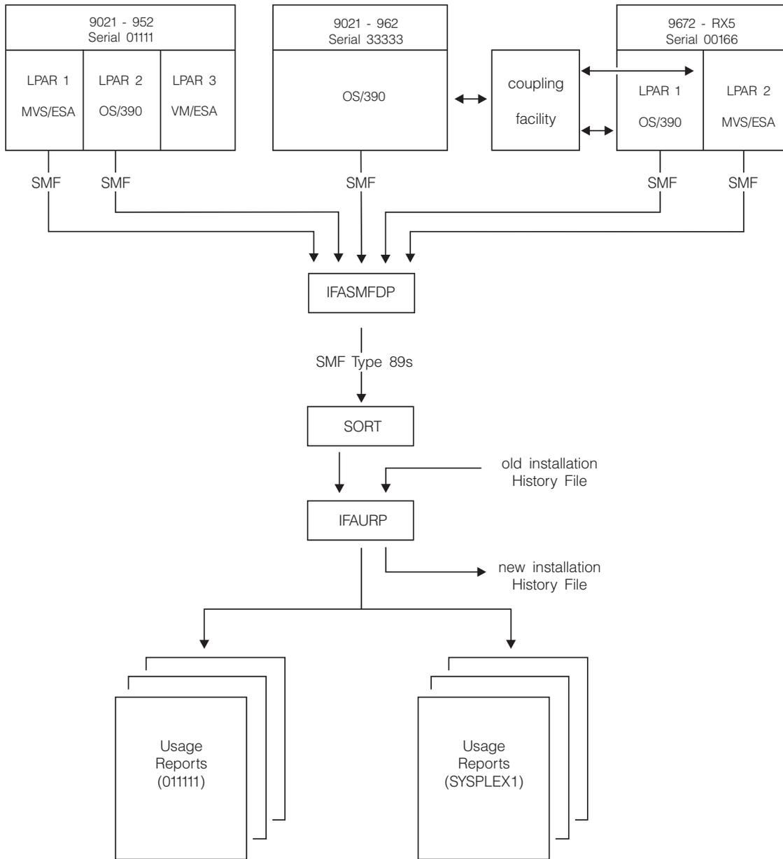
Figure 4. Example of an installation using a single history file for all reporting entities (recommended)
