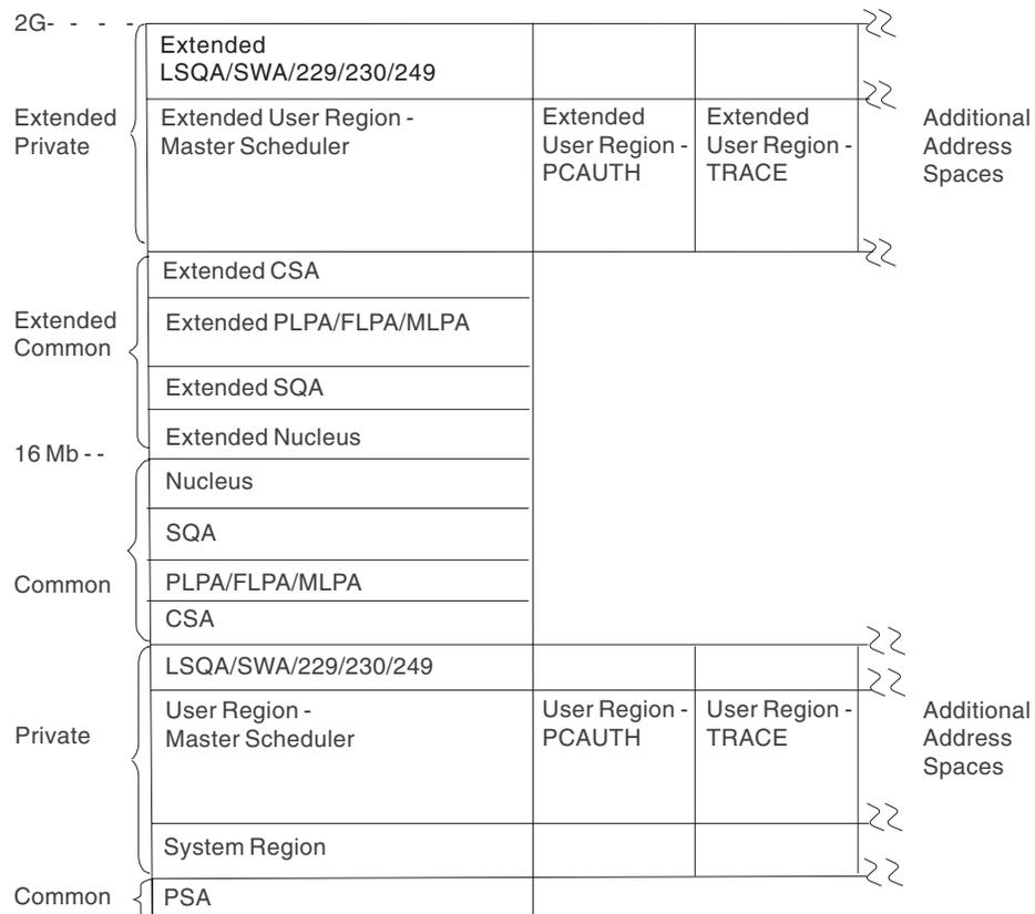
Figure 1. Virtual Storage Layout for Multiple Address Spaces
