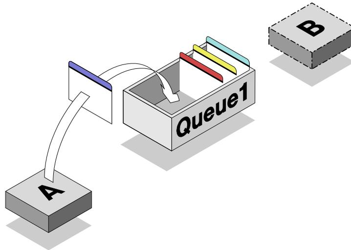
*Figure 3. Either program can be busy or unavailable. In this example, program B is unavailable. The message intended for program B is retained in Queue 1 until the program is available again. (Message queues exist independently of the programs that use them, so both programs could be inactive at the same time; the message on its way from one program to the other is nonetheless retained in Queue 1 until program B is ready for it.)*
