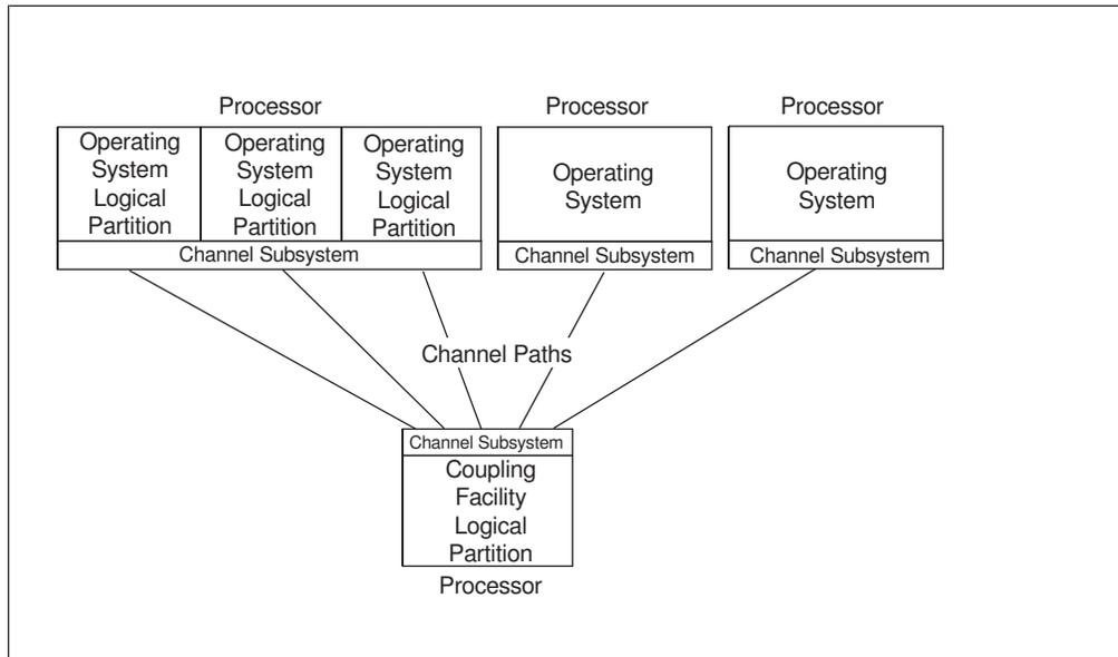
Figure 6. Example of a Sysplex
