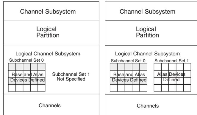
Figure 5. Example of multiple subchannel set configuration
