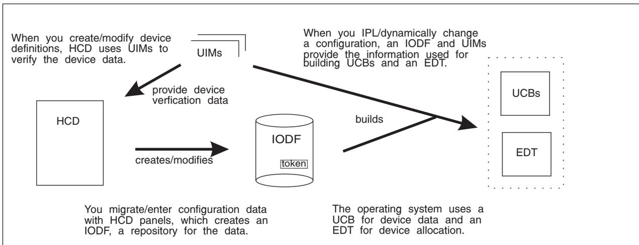
Figure 1. Defining an I/O configuration to the software
