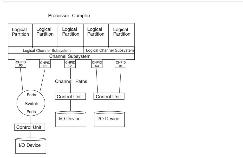
Figure 3. Configuration Example
