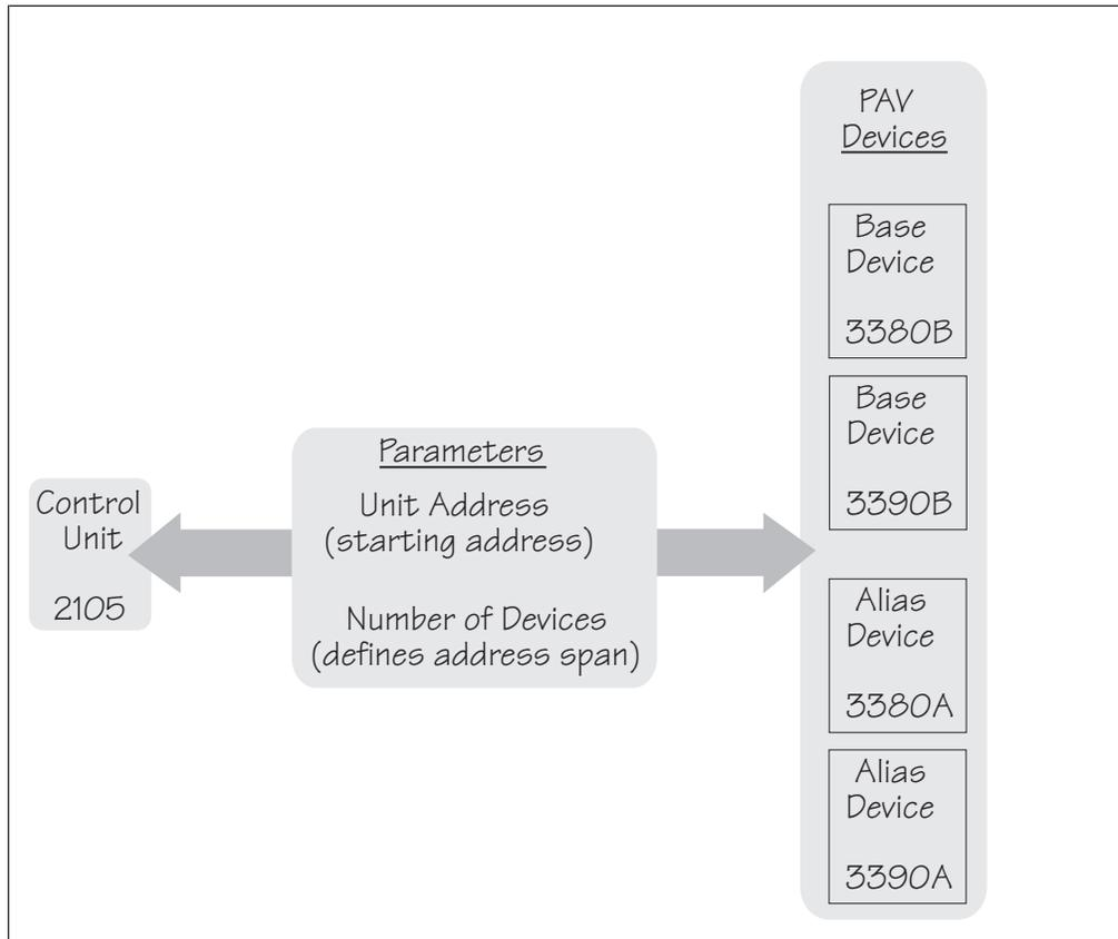
Figure 11. Control Unit - Parallel access volume device relationship
