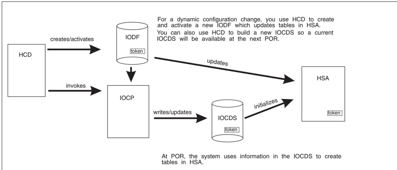
Figure 2. Defining an I/O configuration to the hardware
