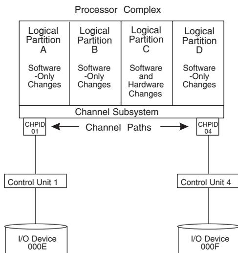
Figure 23. Sample processor running in LPAR mode
